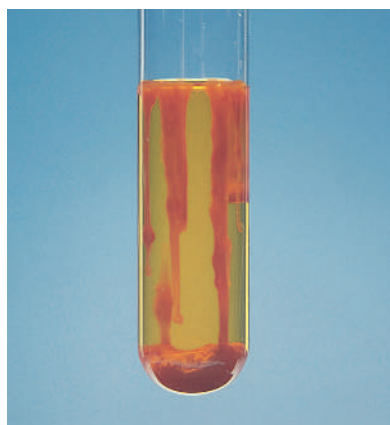
Figure 4.7 Precipitation of iron(III) hydroxide ( \text{Fe}(\text{OH})_3 ). The red, gelatinous precipitate forms when aqueous solutions of sodium hydroxide ( \text{NaOH} ) and iron(III) nitrate ( \text{Fe}(\text{NO}_3)_3 ) are mixed.
