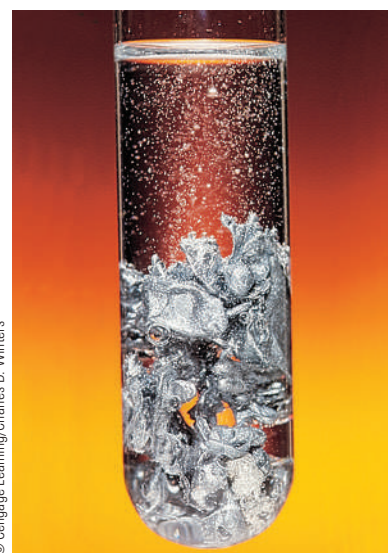
Figure 4.13 Redox reaction of zinc with a strong acid. The zinc atoms are oxidized to \text{Zn}^{2+} ions in solution; the \text{H}^+ ions are reduced to \text{H}_2 molecules.
