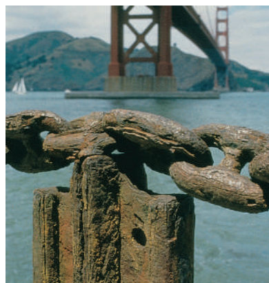
Figure 4.15 Rusting and oxidation number. As iron rusts, its oxidation number changes from 0 in \text{Fe(s)} to +3 in \text{Fe}^{3+} .
