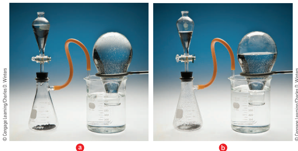
Figure 5.10 Collecting a gas by water displacement. (a) Hydrogen gas is being generated in the flask by an acidic solution dripping onto a metal. (b) When a gas is collected by displacing water, it becomes saturated with water vapor. The partial pressure of \text{H}_2\text{O}(g) in the collecting flask is equal to the vapor pressure of liquid water at the temperature of the system.
