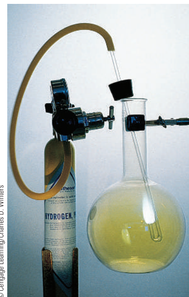
Figure 8.8 An exothermic reaction. Hydrogen, a colorless gas, reacts with chlorine, a pale yellow gas, to form colorless hydrogen chloride gas.
