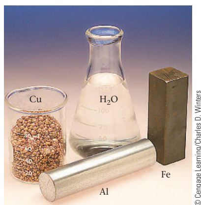
Figure 8.3 Substances with varying specific heats. The metals shown (Cu, Al, and Fe) have specific heats ranging from 0.38 \text{ J/g} \cdot ^{\circ}\text{C} (Cu) to 0.90 \text{ J/g} \cdot ^{\circ}\text{C} (Al). This explains why water warms up and cools down more slowly than a container made of aluminum, copper, or iron.
