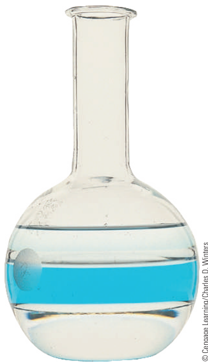
Figure 9.10 Molecular liquids. The bottom layer, carbon tetrachloride ( CCl_4 ), and the top layer, octane ( C_8H_{18} ), are nonpolar molecular liquids that are not soluble in water. The middle layer is a water solution of blue copper sulfate.
