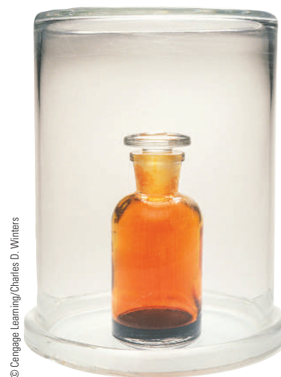
Figure 9.2 Liquid-vapor equilibrium. Under the conditions shown, the bromine liquid and vapor have established a dynamic equilibrium.
