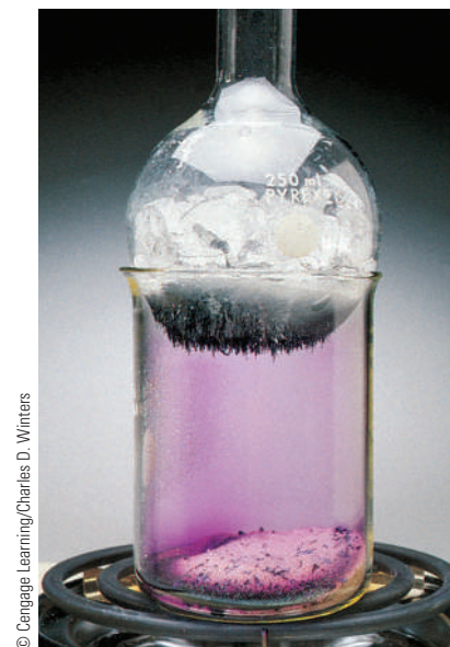
Figure 9.8 Sublimation. Solid iodine passes directly to the vapor at any temperature below the triple point, 114^{\circ}\text{C} . The vapor deposits back to a solid on a cold surface like that of the upper flask, which is filled with ice.
