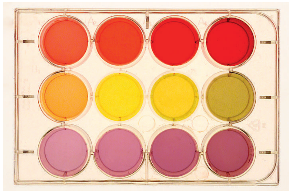
Figure 13.5 pH as shown by a universal indicator. Universal indicator is deep red in strongly acidic solution ( upper left ). It changes to yellow and green at pH 6 to 8, and then to deep violet in strongly basic solution ( lower right ).
