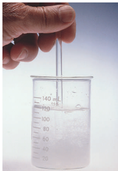
Figure 13.13 Sodium chloride solution. When the NaCl is completely dissolved, the solution will contain only Na + , Cl - , and H 2 O, and it is neither acidic nor basic.
