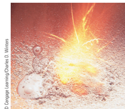
Figure 13.12 Hydride ion–water reaction. As water is dropped onto solid calcium hydride, the hydride ion ( \text{H}^- ) reacts immediately and vigorously to form \text{H}_2(\text{g}) (which is ignited by the heat of the reaction) and \text{OH}^- .
