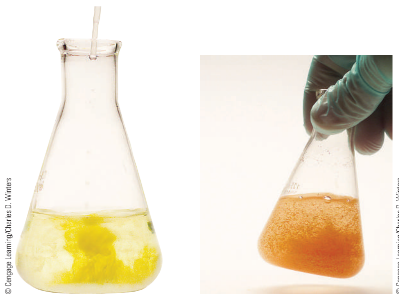
Figure 15.6 Titration of \text{Cl}^- with \text{Ag}^+ , using \text{CrO}_4^{2-} as an indicator. \text{AgCl} (cream color) comes down first, then \text{Ag}_2\text{CrO}_4 (red) precipitates.
