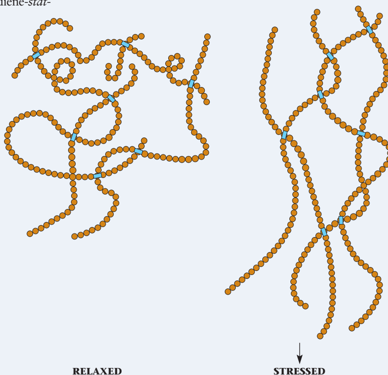
Figure B Pulling down on the elastomer. The chains become oriented in the elongational direction, lowering the entropy of the system.
