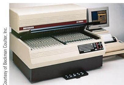
Figure 18.6 A liquid scintillation counter. This instrument is used to detect radiation and measure disintegrations per minute quickly and accurately.
