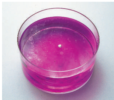
Figure 20.7 Reaction of sodium with water. When a very small piece of sodium is added to water, it reacts violently with the water. The \text{OH}^- ions formed in the reaction turn the acid-base indicator phenolphthalein from colorless to pink.
