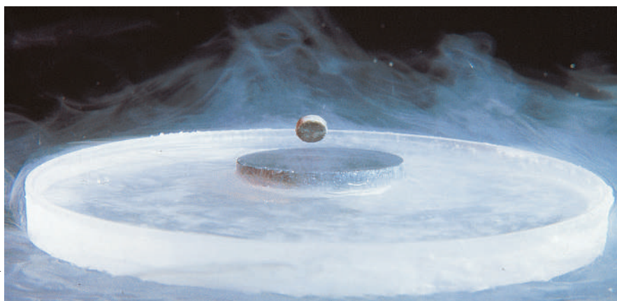
Figure 20.11 A superconductor. A pellet of superconducting material, previously cooled to 77 K with liquid nitrogen, floats above a magnet.
