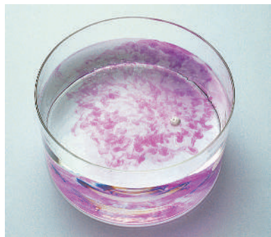
Figure 20.7 Reaction of sodium with water. When a very small piece of sodium is added to water, it reacts violently with the water. The \text{OH}^- ions formed in the reaction turn the acid-base indicator phenolphthalein from colorless to pink.
