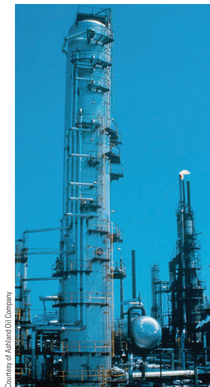
Figure 22.4 Petroleum distillation. (a) A distillation tower at a petroleum refinery. (b) A diagram showing the boiling points of the petroleum fractions separated by distillation.
