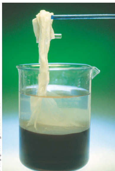
Figure 23.3 Nylon. Nylon can be made by the reaction between hexamethylenediamine, \text{H}_2\text{N}-(\text{CH}_2)_6-\text{NH}_2 , and adipic acid, \text{HOOC}-(\text{CH}_2)_4-\text{COOH} . It forms at the interface between the two reagents.
